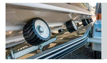
**LEFT** The 635 rides on a galvanised steel, twin-axle, braked, multiroller trailer from DMW.
